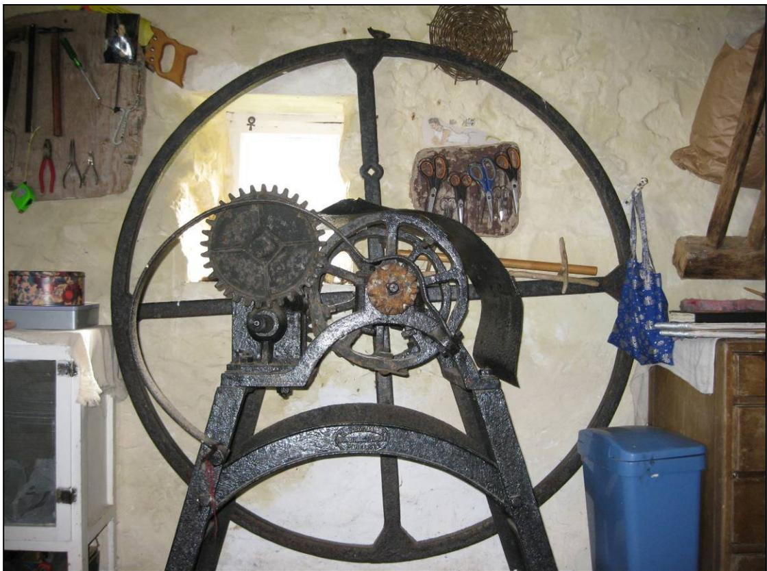
**Photo 20:** A well-preserved gorse chaff cutter in a building on Bardsey Island. This particular cutter was powered by horses rather than by a water wheel.
